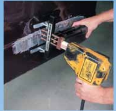
The dent is levered out using only the required amount of pull to leave a flat surface. The Dent Killer is then rotated around the weld to release the electrode, leaving a flat, workable surface.
